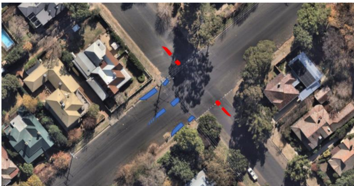
Figure 4: Additional pedestrian refuges (shown in red) are proposed at the White Street and Upper Street intersection in East Tamworth.
