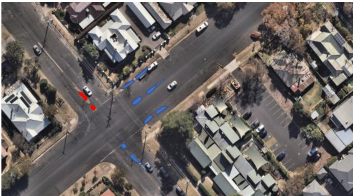
Figure 3: An additional Pedestrian refuge (shown in red) is proposed at the White Street and Carthage Street intersection, East Tamworth
